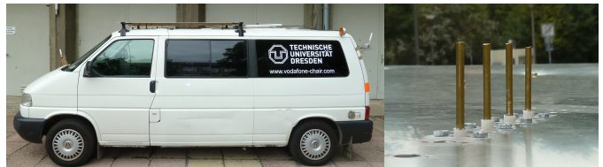
Fig. 5. The Volkswagen T4 van on the left hand side and zoomed into the antenna array on the roof on the right hand side.
