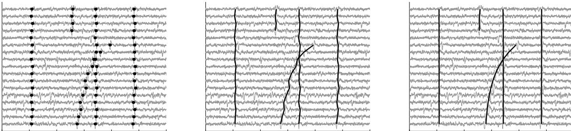
Figure 2. Sample results from the three steps of the algorithm. To the left, the detection is shown. The middle figure displays the five resulting tracks. To the right, parametric models have been fitted to these tracks.
