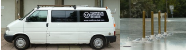
Fig. 5. The Volkswagen T4 van on the left hand side and zoomed into the antenna array on the roof on the right hand side.
