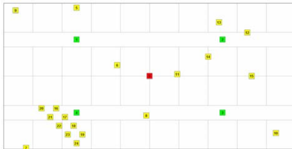
Figure 4.2: Baseline relay deployment in indoor scenario
